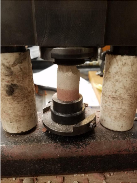
FIGURE 9 CORE SAMPLE UNDER UCS TEST MACHINE
