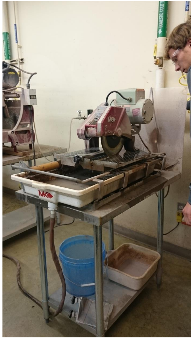
FIGURE 7 CORE CUTTING ON TILE CUTTER
