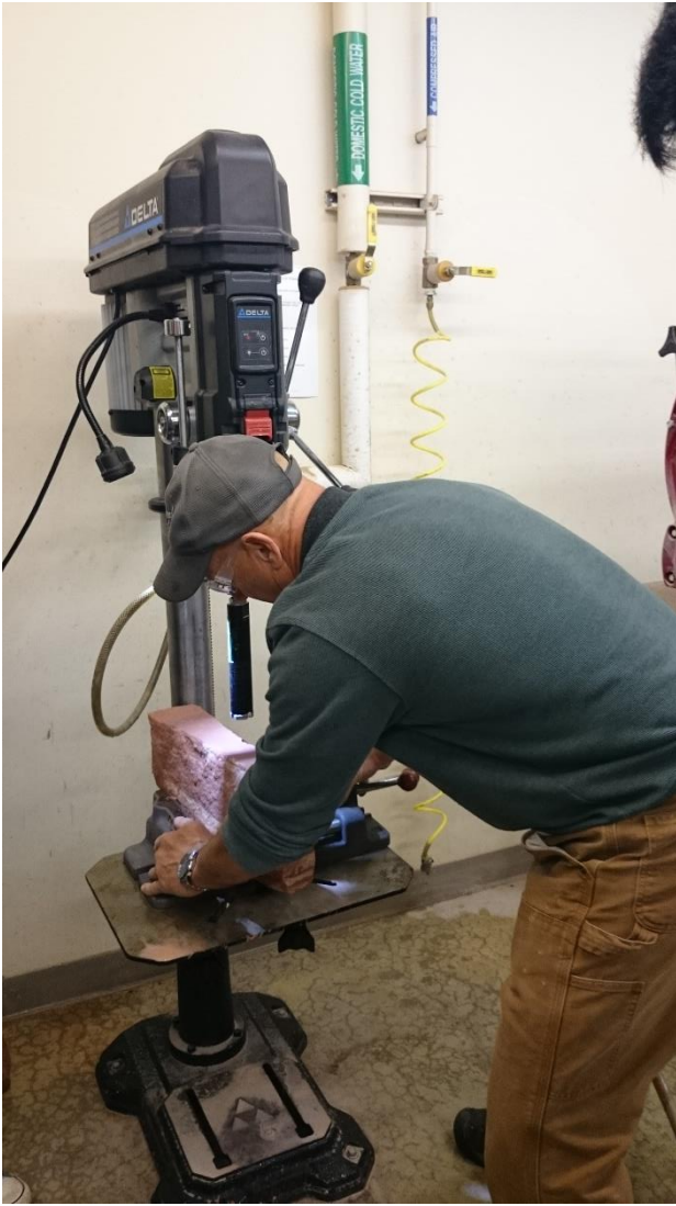
FIGURE 6 CORING ON DRILL PRESS
