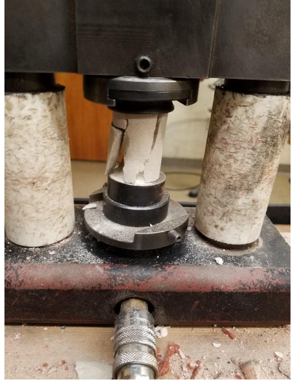
FIGURE 10 PERFECT 45 DEG FRACTURE PLANE
