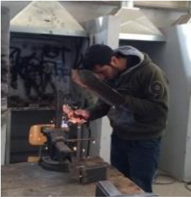
Figure 21: Soudage de la structure
