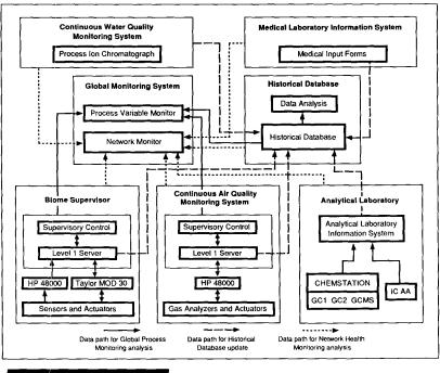
FIGURE 1. Nerve System Architecture
