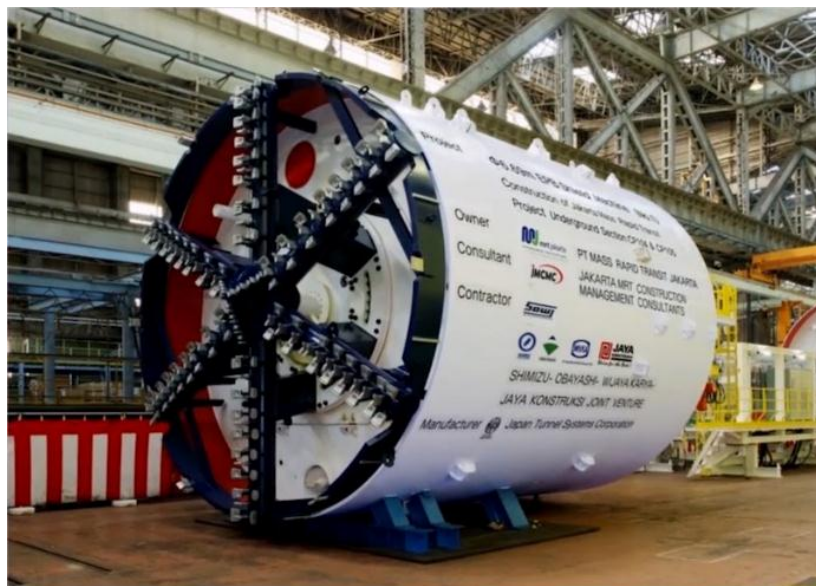
Gambar 2.4 Tunnel boring machine
